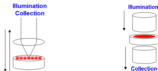
Fig. 1 Geometry of the transmission measurement (right) as opposed to the backscattering mode (left).
