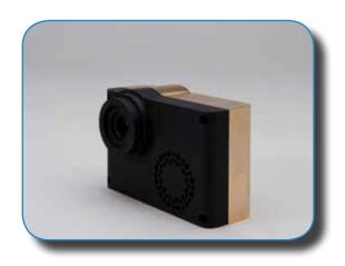
PPD detectors are compact and include all electronics required to detect single photons with picosecond accuracy. The module contains a wide bandwidth GHz pre-amplifier, picosecond timing constant fraction discriminator and regulated high voltage supply all in one compact, fully integrated package.
